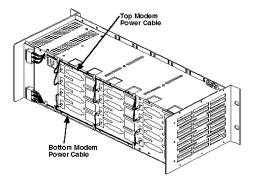
Figure 2-2. Modem Power Connection
